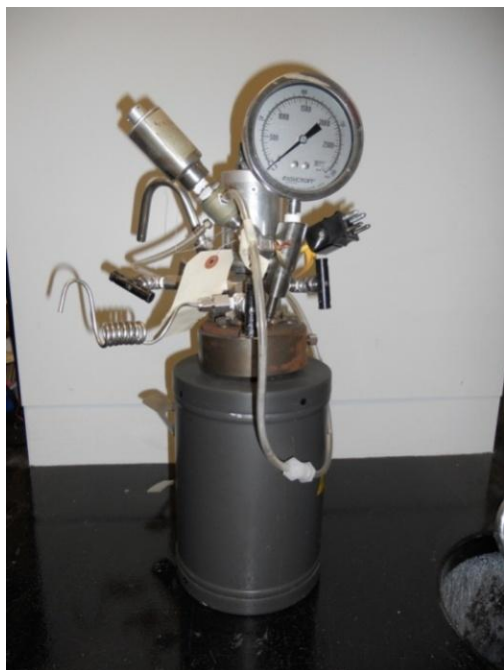
Figure 2. Autoclave to study hydrothermal stability and scale inhibition
