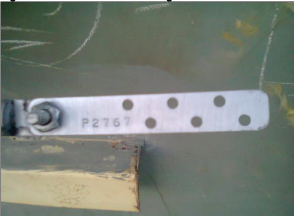
Figure 11. The scale coupon from the exit of the heat exchanger
