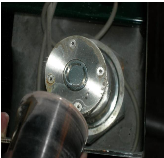
Figure 7. RTM an online scale rate monitoring device
