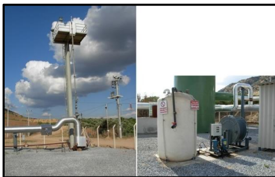
Figure 1: Bundled chemical feed equipment package showing pump skid, insulated tank, capillary tubing, and wellhead lubricator assembly.
