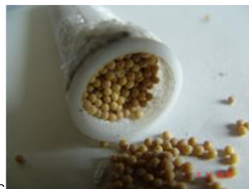
Figure 4: Wairakei prolonged aging; A – aging tank; B – no scaling after 186m 3 of 50°C aged water passed through a column containing 1mm diameter ceramic beads; C – column blocked after passing 15m 3 of water containing excess monomeric silica
