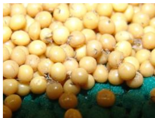
Figure 5: Ceramic bead showing trapped debris
