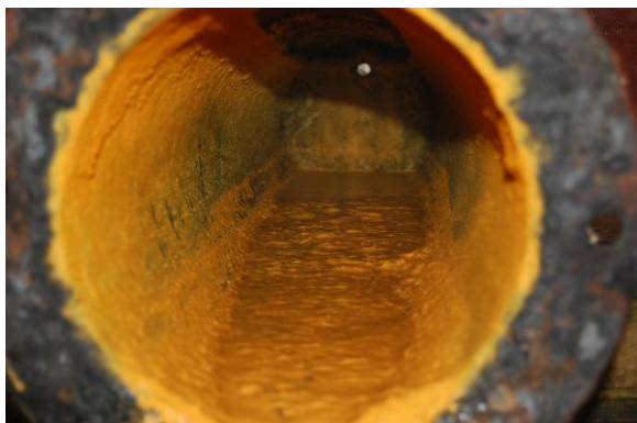
Figure 11. Photo of the retention vessel with the slurry deposits after the testing
