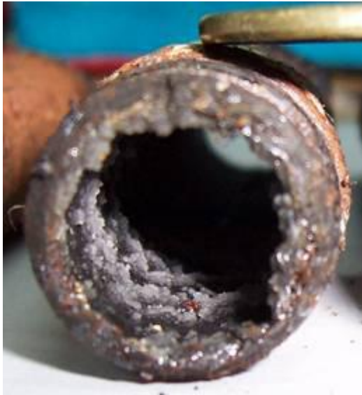
Figure 5. Sample of pipe with thickest deposit of soft silica.
