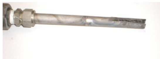
Figure 9: Photo of damaged acid injection tube.
