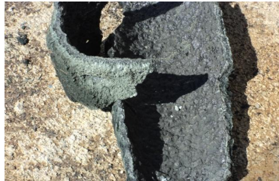
Figure 4: Photo of Thick scale formation at separator brine outlet.
