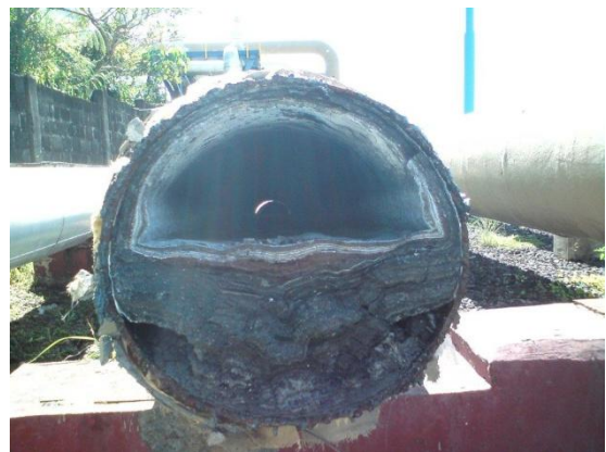
Figure 11 More evidence of low flow conditions possibly as a result of the reduction in the capacity of the injection wells.
