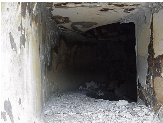
Figure 16 Silica scaling at the inlet of a separator.
