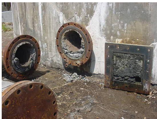
Figure 5 Silica scales on Atmospheric Flash Tanks
