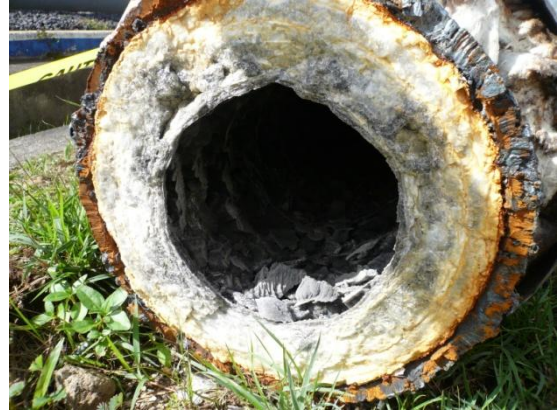
Figure 10 Silica scaling possibly due to cooling of the brine as a result of the long distances.
