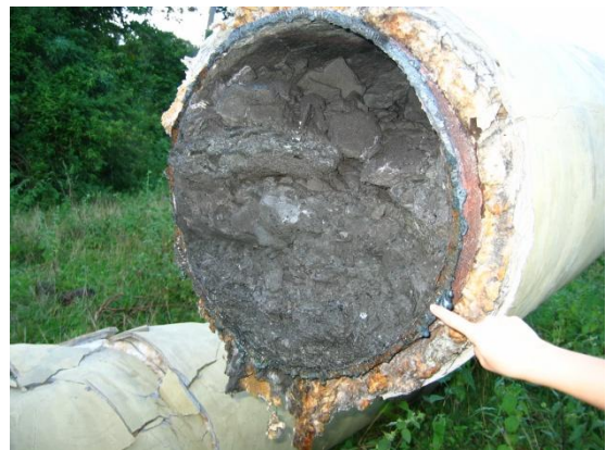
Figure 12 Accumulation of scale and debris were also observed at low points in the brine lines.
