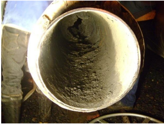
Figure 15 Silica scaling along a two-phase line where a dry-steam well mixes with a two-phase well.
