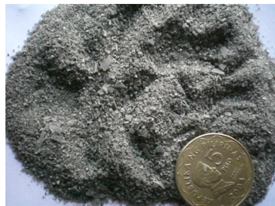
Figure 14 Silica scales that eroded the 3" pre-heating line of Kap34.
