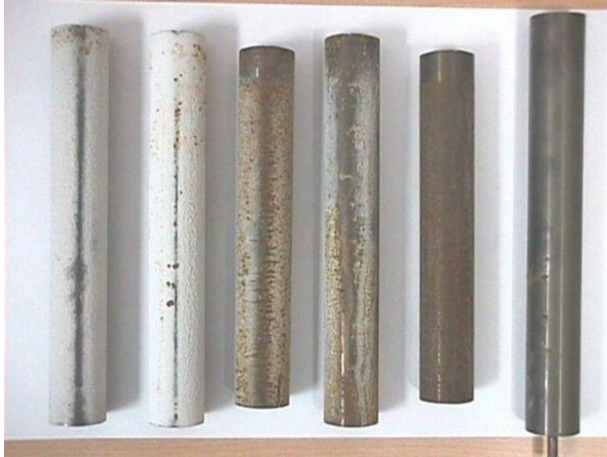
Figure 7: Silica scaling under controlled hydrodynamic and colloid particle size. From L to R: large particles - slow velocity, large particles - fast velocity, medium particles - low velocity, medium particles - fast velocity, small particles - low velocity and small particles - fast velocity.
