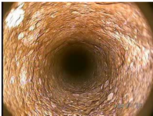
(a) look of a downhole drilled by rotary bit
