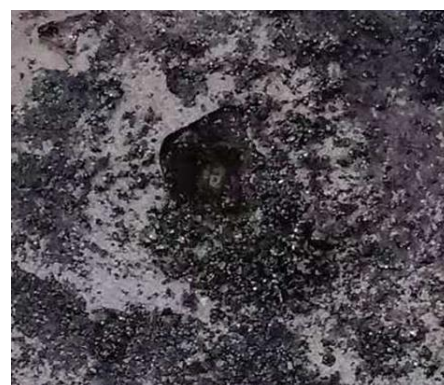
(b) Combination of fusion and spallation with water cooling
