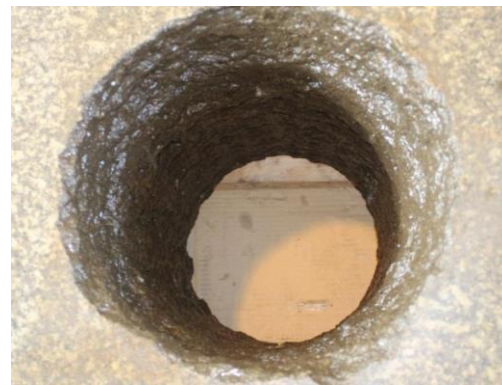
(b) look of a hole drilled by the EI bit in OBM
