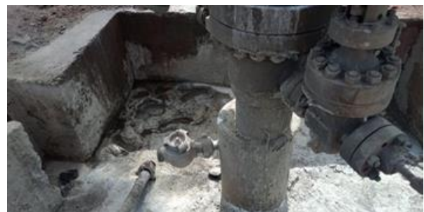
4. After conducting the squeeze operation and pumping 4m 3 of slurry
