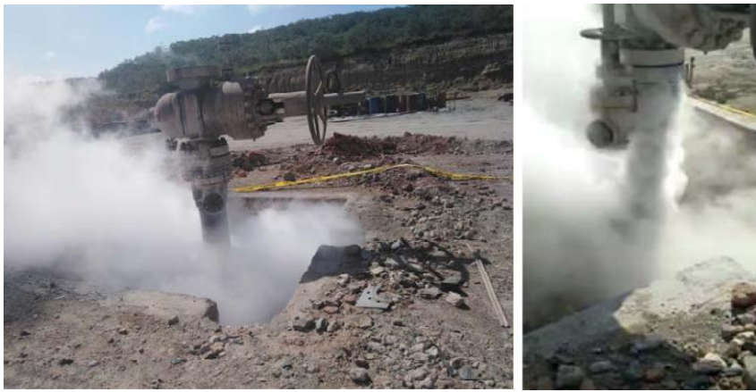
FIGURE 3: Steam leakage at later stages of development.
