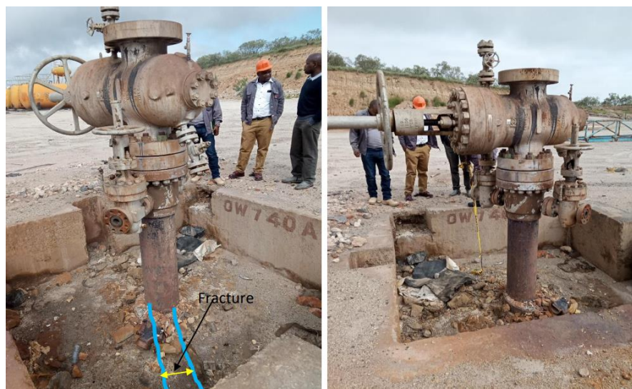
FIGURE 2: Situation at well OW-740 at the initial stages of steam leakage development (July 2019)
