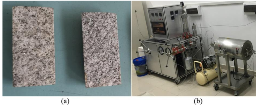
Figure 1. (a) One split granite rock sample and (b) Fluid flow-through experiment device.
