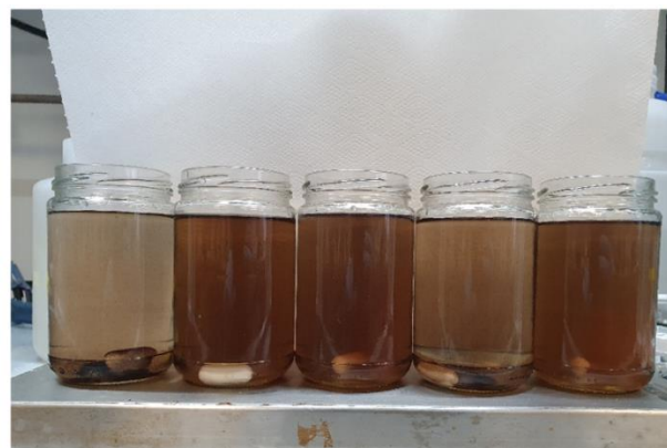
Figure 4: Results of PbS dispersion test (above). In the pictures (t=0 and t=2h respectively), from left to right: Blank, Competitor, SPE2122 A, SPE2122 B, SPE2122 C
