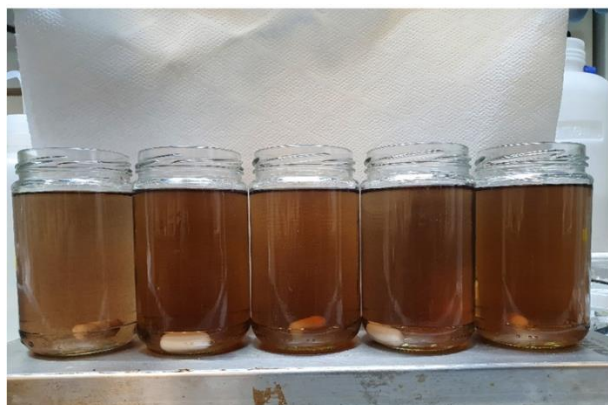
Figure 4: Results of PbS dispersion test (above). In the pictures (t=0 and t=2h respectively), from left to right: Blank, Competitor, SPE2122 A, SPE2122 B, SPE2122 C
