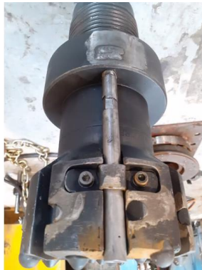
Figure 12: Modified hammer drill bit with HPWJ nozzle
