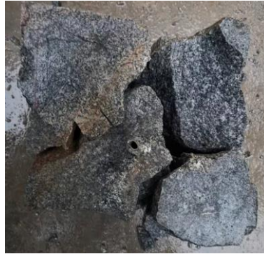
Figure 9: Samples after the test with extreme low temperature fluid
