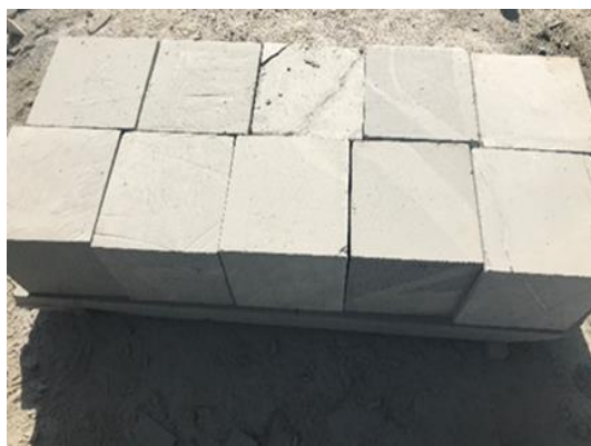
Figure 2: Prepared samples for laboratory hydraulic fracturing tests
