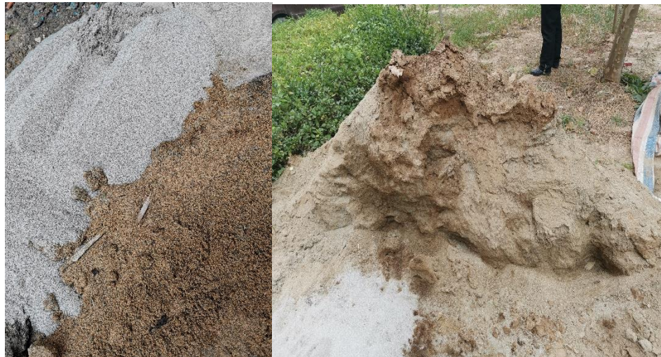
Fig.3-2 Sand production in geothermal well site
