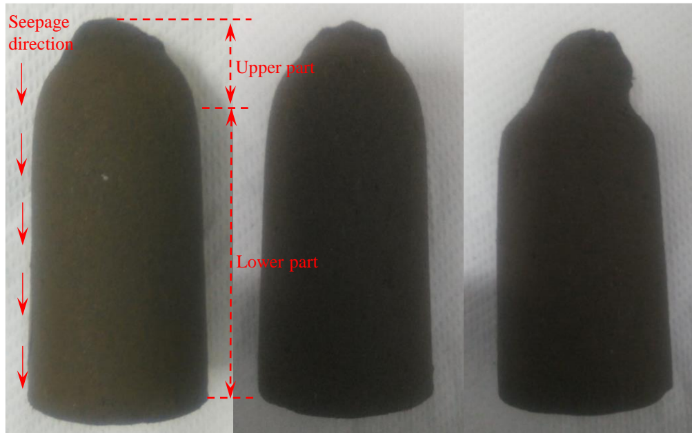
Figure 9 Photos of damaged samples after seepage experiment
