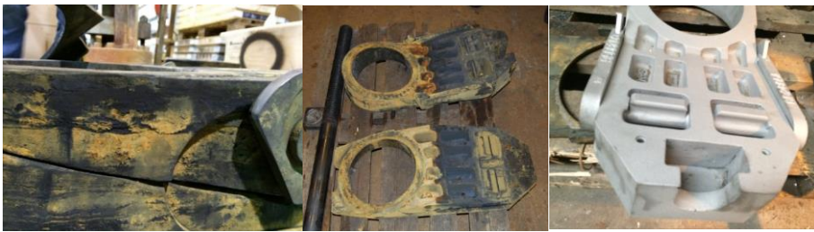
Figure 3: Gate and segment. a) Gate segments showing distortions b) Back side of gate and segment c) Gate after sandblasting.
