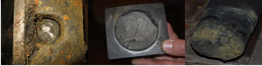
Figure 2: Broken parts of the stem. From left to right: Broken stem shown in gate when dismantling the valve, broken bottom part of stem after cleaning, end of broken stem.
