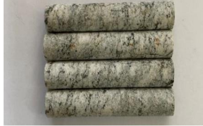
The cylindrical specimen used to determine the coefficient of thermal expansion
