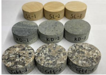
Disc sample used for measuring thermal conductivity
