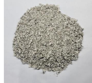
Powder sample used to determine the specific heat capacity
