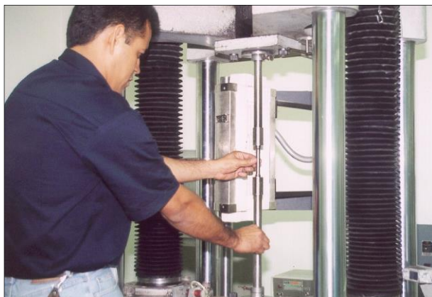
Figure 3: Placement of the sample in the special equipment for the tension test at different temperatures.
