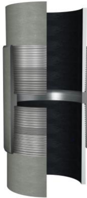
Figure 10: Connection TXP BTC that was used in slotted liner of 7", with special coupling torque shoulder, design provides high torque and compression capacity for rotating applications.
