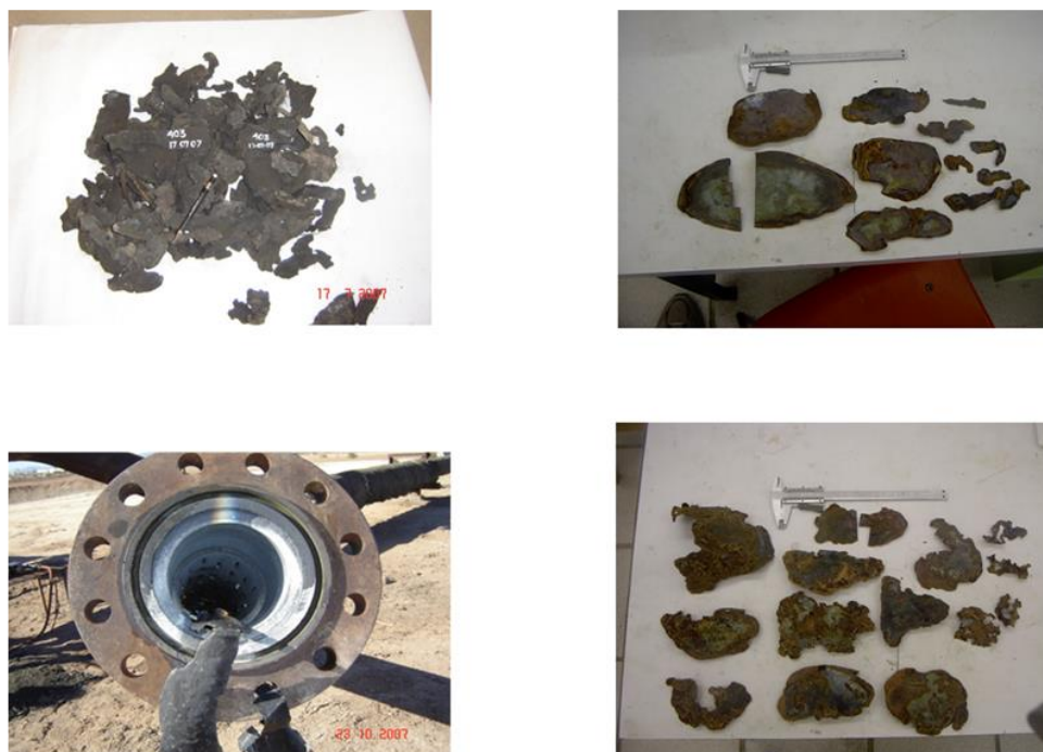
Figure 6: Steel pieces in the head of the well due to the corrosion phenomenon of CO 2
