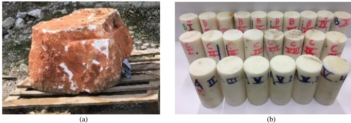
Figure 1: (a) Large marble block representative of the deep reservoir in Kızıldere, and (b) Cored and polished marble samples for laboratory experiments.
