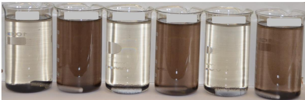
Figure 5: Efficiency of lead sulfide dispersing of different inhibitors at 50 mg/l after 60 min of settling time (from left to right: blank, polycarboxylate 2, phosphonate 5, polycarboxylate 1, phosphonate 1, polycarboxylate 5).
