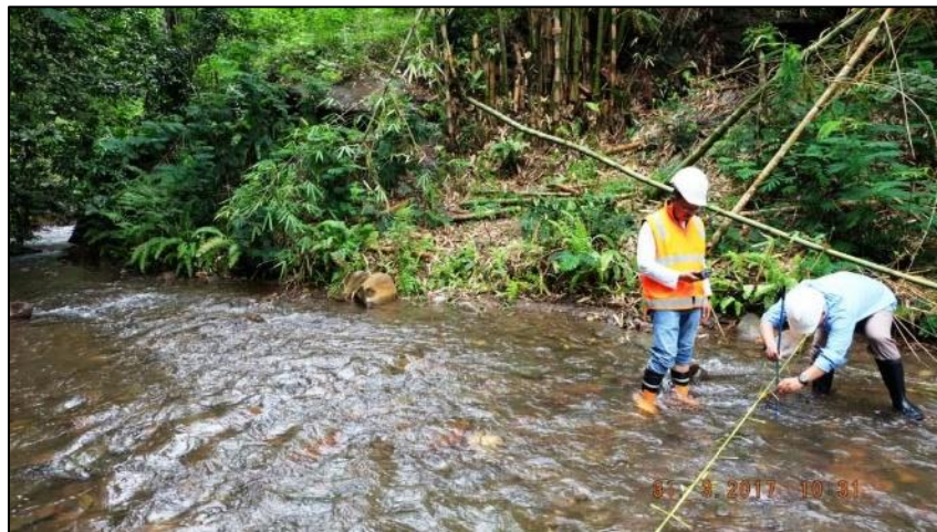
Figure 6. Flow rate measurement on of the rivers. The flow rate is adequate but has a pH of 2.
