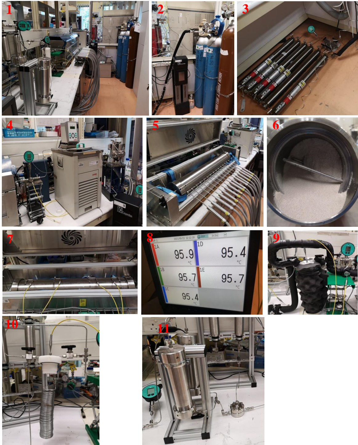
Figure 3 Pictures of the geothermal heat mining setup. 1: whole image of the setup; 2: CO 2 tank and pump; 3: CO 2 accumulators; 4: cooling circulator and inlet; 5: sandpack, multipoints thermocouples and heating cabinet; 6: multipoints thermocouple inside the sandpack; 7: surface thermocouple on the sandpack; 8: thermocouple data logger; 9: outlet and heat exchanger; 10: coil inside the heat exchanger; 11: flashing cylinder.
