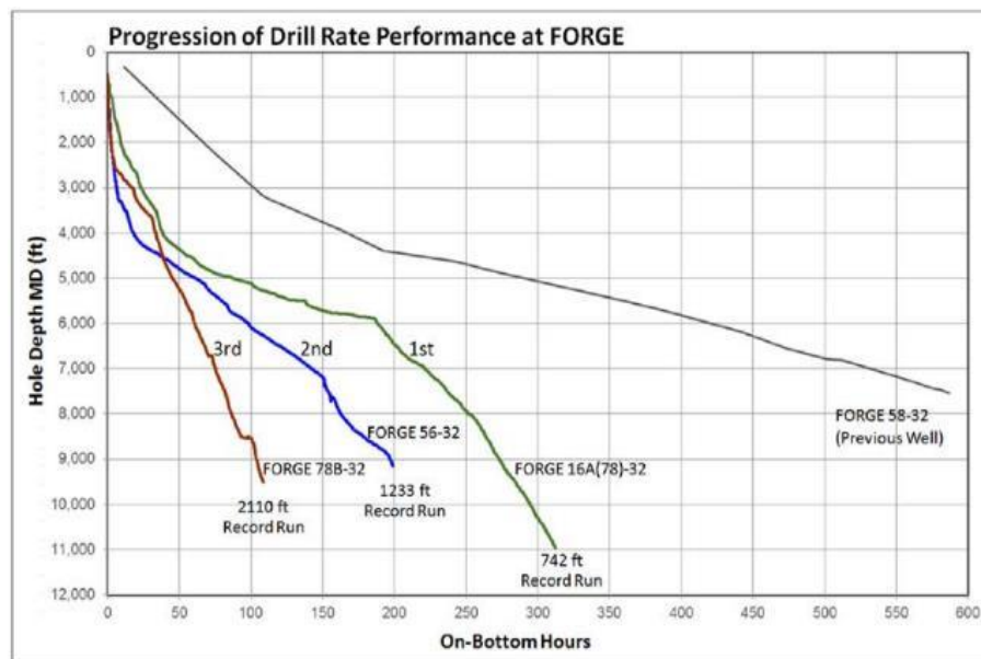
Figure 5: On-bottom rotating hours in sequentially drilled wells at Utah FORGE (Dupriest and Noynaert (2022)).
