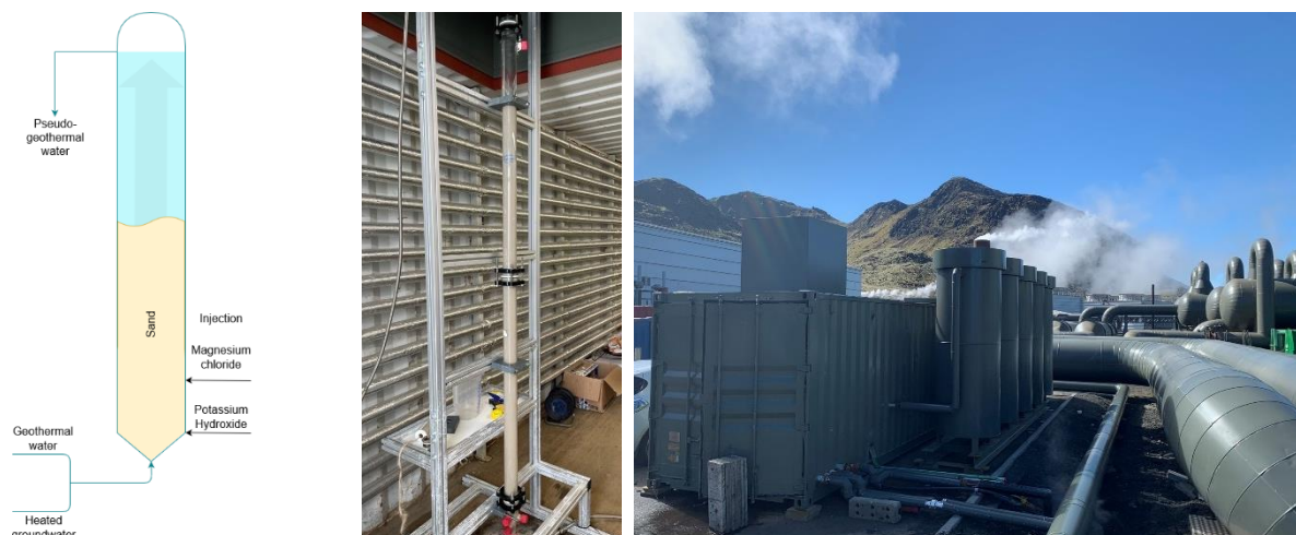
Figure 2: Left: A schematic of the FBR used in the flowthrough experiments showing the inlet streams of geothermal water and heated groundwater, dosing connections and the resulting pseudo-geothermal water after passing through the FBR. Middle: The glass FBR column during operation. Right: Experimental facilities located at the Hellisheiði power plant.
