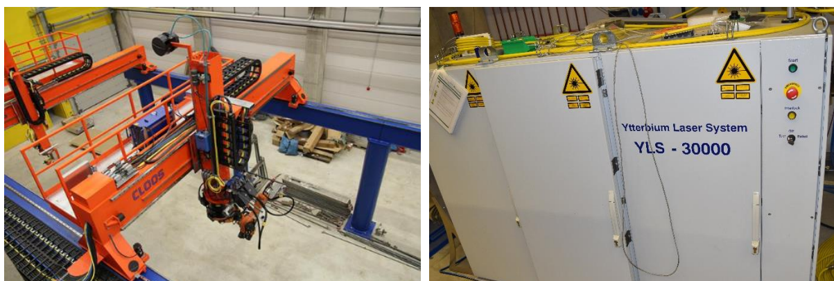
Figure 4: Large gantry system for laser positioning (left) and 30 kW high-power laser (right) at Fraunhofer IAPT facilities.
