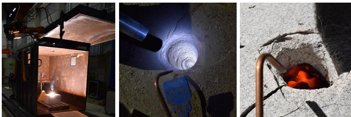
Figure 5: Experimental set-up in a press container and first drilling results in a sandstone or granite block.
