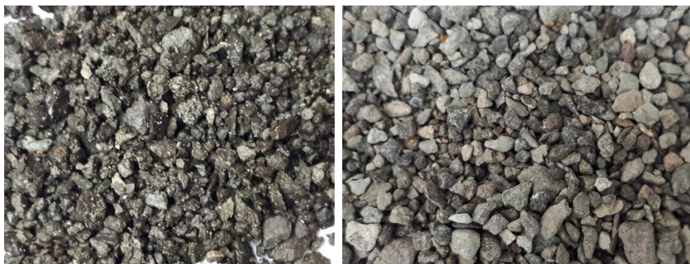
Figure 8: Dieng - Pilot Plant Packed bed drill cuttings in inlet and outlet for hot injection process (MICK 2021).
