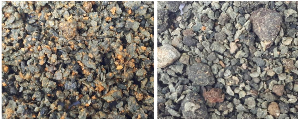
Figure 7: Dieng - Pilot Plant - Packed bed drill cuttings in inlet and outlet for ORC process (MICK 2021).
