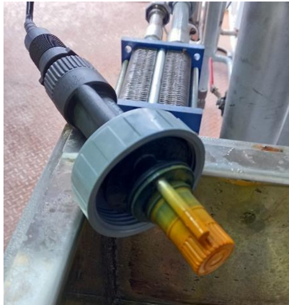
Figure 2: Dieng - Pilot Plant - Contaminated pH electrode, As 2 S 3 84%, Sb 2 S 3 16%. (MICK 2021).
