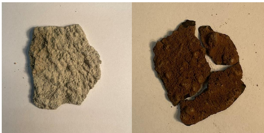
Figure 1: Two pieces of cement lining from storage tanks in the district heating system of the Reykjavík capital area. The piece of cement lining on the left is from a storage tank which is fed with hot water from the Nesjavellir power plant. The piece of cement lining on the right is from a storage tank fed with hot water from the Hellisheiði power plant. An XRD analysis confirms that both cement lining pieces have a layer of amorphous magnesium silicate scaling precipitated on top of them. However, in the piece of lining from the Hellisheiði storage tank the magnesium silicate contains a significant amount of iron, 24% of the weight of the sample, as is also evident from the strong red color of the sample.
