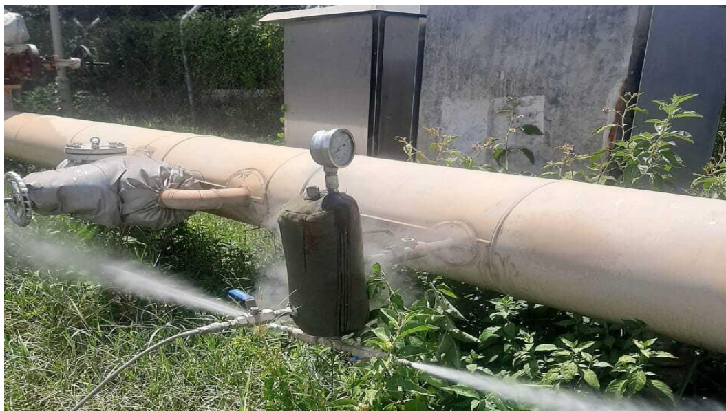
Figure 2: Webre Separator connected to the brine line of one of the re-injection streams
