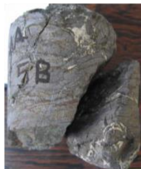
Figure 5: Calcite in veins, TO-1 (1500-1503 m)
