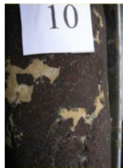
Figure 6: Calcite in vesicle, TO-1A (1182 - 1186 m)
