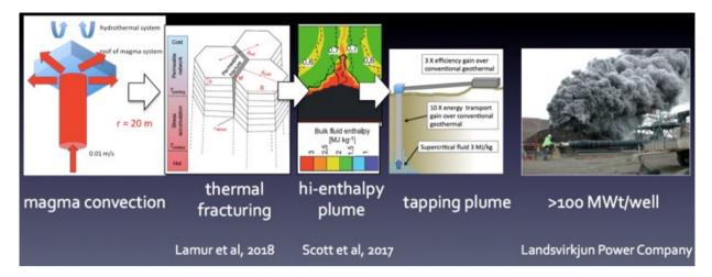
Fig. 8: Idealized scenario for magma-sourced geothermal energy.
