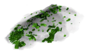
Figure 2: X-ray tomograph of rhyolite magma quenched at 2100 m depth in IDDP-1 and recovered by circulating drilling fluid. False-color green crystals, mostly plagioclase feldspar, float in transparent melt (now glass) "space". Long dimension of chip is 3mm. Sample provided by Landsvirkjun (National Power Company of Iceland) and imaged by imaged by Fabian Wadsworth at Munich University working with Elodie Saubin, University of Canterbury and Ian Schipper, University Wellington, New Zealand.
