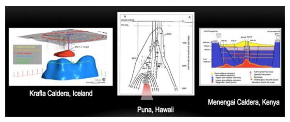
Figure 1: (L) Plausible model (JW Catley, Reykjavik University) for rhyolitic (red) and basaltic (blue) magma beneath Krafla Caldera (red circle). Geothermal wells (~40) are gray. Planned site and target of KMT-1 are also shown. Two wells penetrated magma and four others may have come close based on temperature and gases. (M) Dacite magma encountered under the lower east rift of Kilauea volcano (Teplow et al, 2009). (R) Syenite magma body centered under Menengai Caldera (Mbia, et al, 2015).
