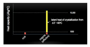
Figure 3: Comparison of the heat capacity of solid rock, the main component and storer of heat of a hydrothermal reservoir, with the effective heat capacity of rhyolitic magma within its crystallization interval.
