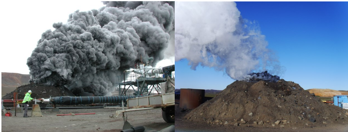
Figure 7: Steam from IDDP 1, initial discharge on the left and superheated steam after 30 minutes discharge on the right
