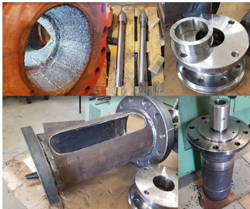
Figure 11: Orifice valve manufacturing process.
