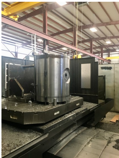
Figure 7: 90° angle wellhead spool being milled at Triple J.
