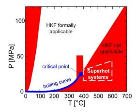
Figure 4. Range of applicability (white area) of the widely used HKF model for geofluid thermodynamics.
