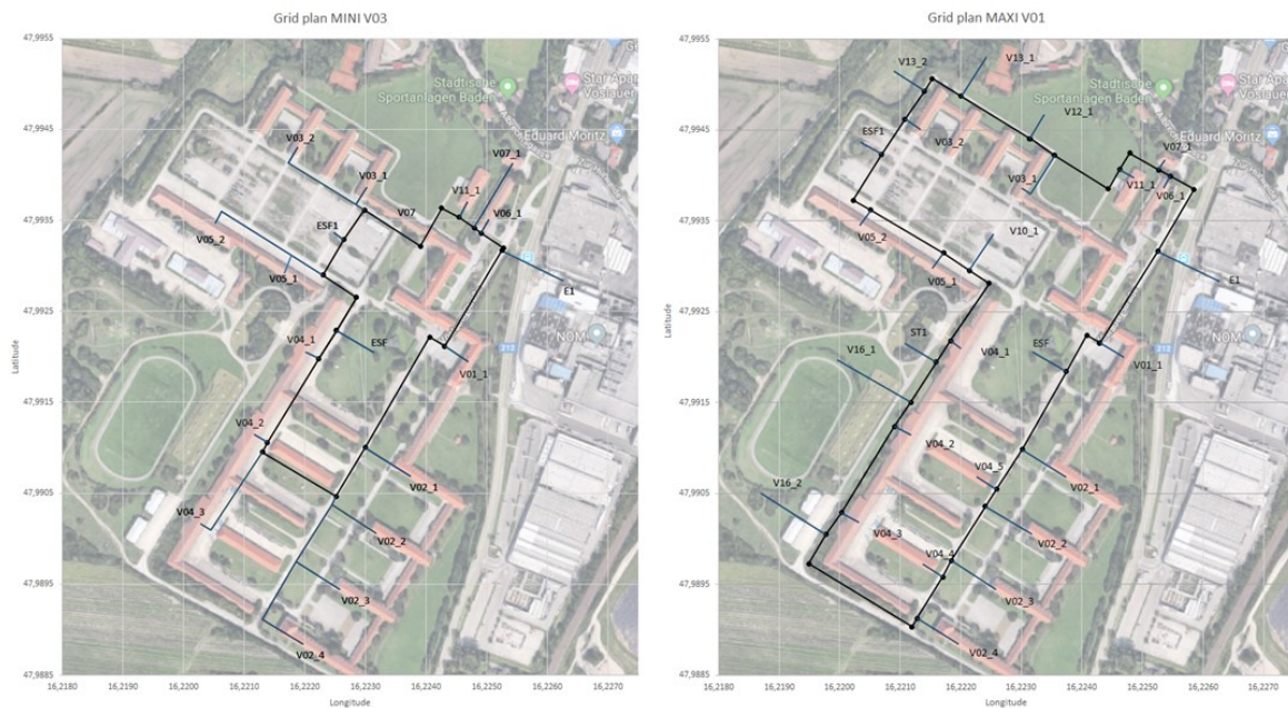
Figure 6: Network of the LTHC grid for scenario MINI and MAXI.
