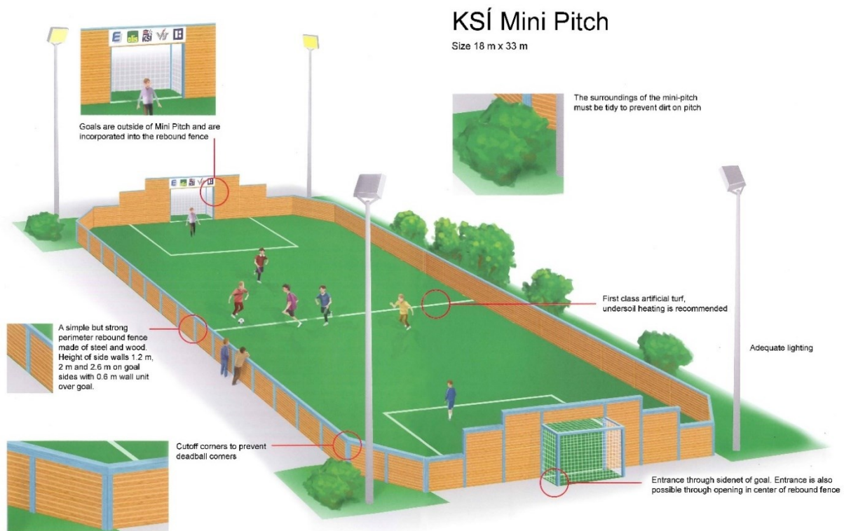
Figure 3: Drawing of a typical mini-pitch, with necessary technical systems, as advocated for in the KSÍ mini-pitch project (modified from KSÍ, 2004).
