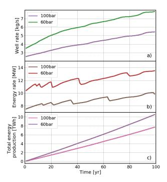
Fig. 8 Time evolution of well rate (a), energy rate (b) and total energy production (c) for two single production well simulations with bhp set to 60 and 100 bar
