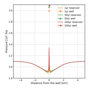
Fig. 4 Reservoir and well pressure along the horizontal line cutting through the middle of the open well section (2150 m depth) after 1, 50 and 100 years of cold water injection with rate=3.2 kg/s
