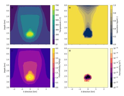
Fig. 2 Temperature (a), liquid saturation (b), fluid enthalpy (c) and rock permeability (d) after 2700 years of magma cooling
