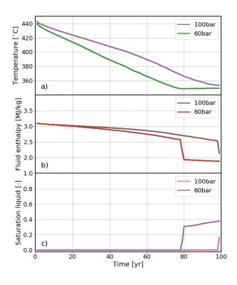
Fig. 7 Time evolution of bottom hole temperature (a), fluid enthalpy (b) and liquid saturation (c) for two single production well simulations with bhp set to 60 and 100 bar
