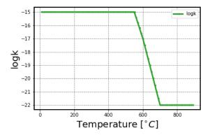
Fig. 1 Logarithm of permeability as a function of temperature for basaltic rocks from Hayba and Ingebritsen (1997)
