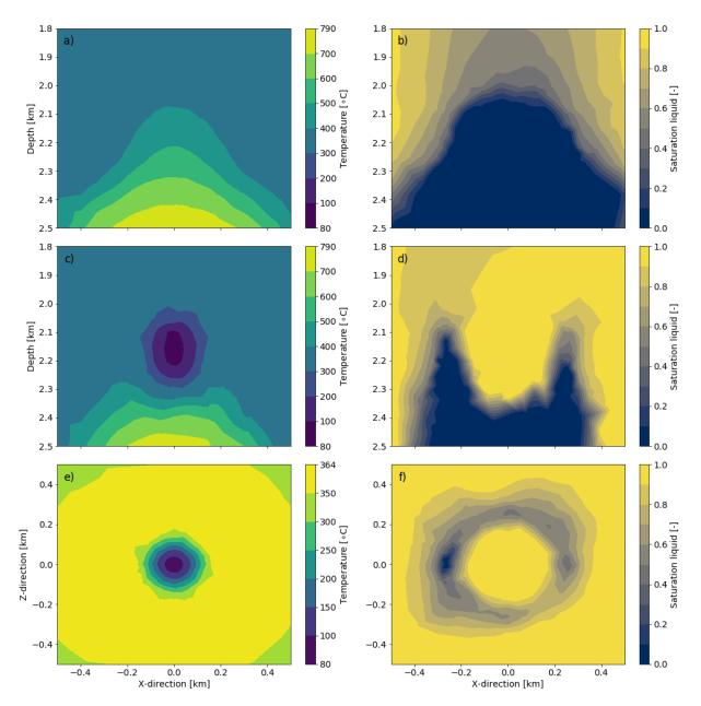
Fig. 3 Temperature (a) and liquid saturation (b) prior to injection, and after 100 years of cold water injection with rate=3.2 kg/s in the vertical slice along the well (c,d) and the horizontal slice (e,f) through the well middle
