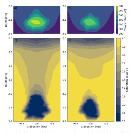
Fig. 6 Temperature (a) and liquid saturation (c) prior to production and (b,d) after 100 years of fluid production with a bottom hole pressure of 100 bar in a vertical slice through the model center
