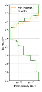
Fig. 5 Permeability along the vertical line through the model center after 100 years of cold water injection with rate=3.2 kg/s compared to natural geothermal system evolution
