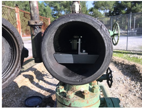
Figure 2: a set of 7 coupons installed in a dedicated rack for corrosion study installed in a Cazaux oil well (Source: Vermillon).
