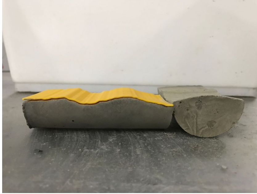
Fig. 3 The concrete specimens of B (Long side JRC 10-12)
