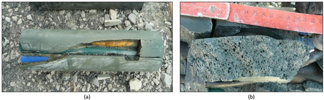
Figure 2: (a): incomplete backfilling, partially filled with water, (b): porous backfilling
