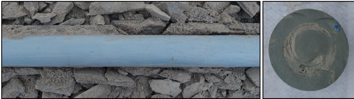
Figure 10: left: dismantled backfilling built in sand formation. right: selected cross-section of the same backfilling.
