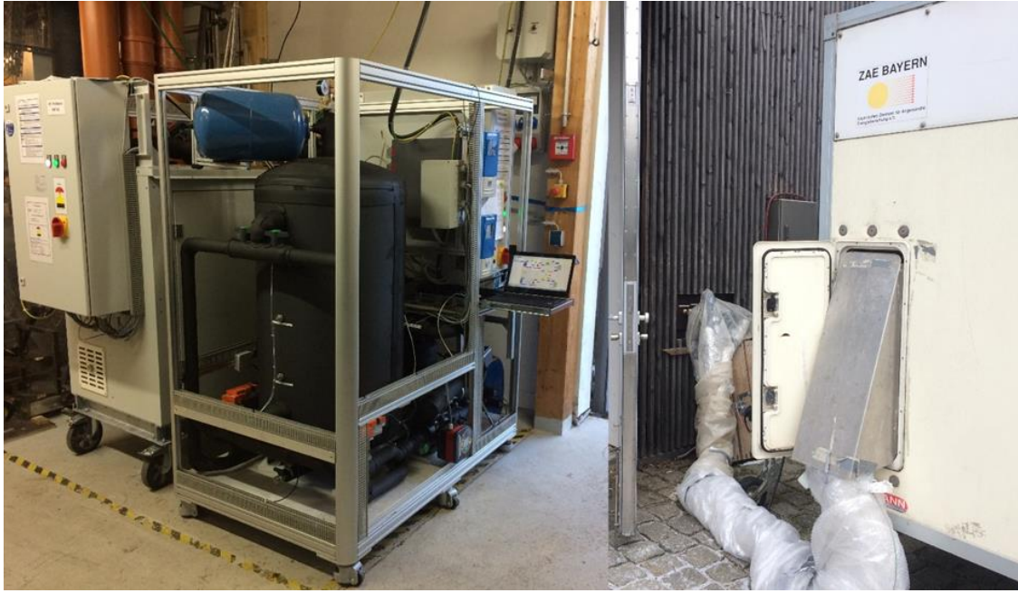
Figure 3: At the ZAE Bayern developed and built up E-BHE (left side) with a connected high precision TRT unit of ZAE Bayern (right side).
