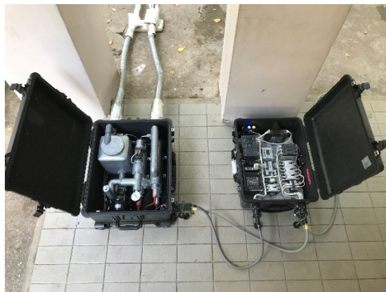
Figure 8. TRT measurement in Bangkok GSHP site
