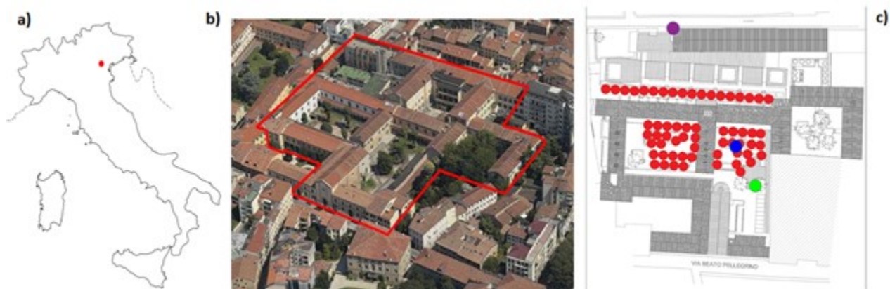
Figure 1: a) The location of the test site in Padua, Italy; b) The overview of the complex of building constituting the test site and c) the borefield layout (in red) with the position of the monitoring wells (in purple, blue and green).
