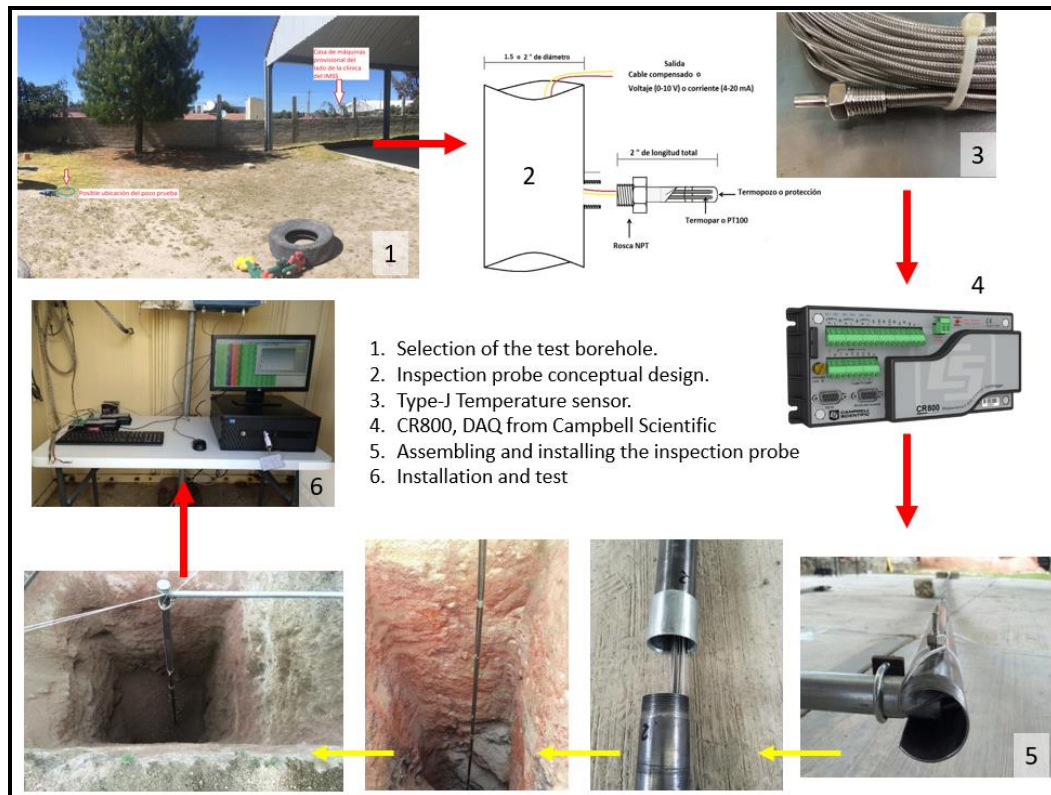
Figure 5: General diagram to measurement the ground temperature profiles (From presentation AGM 2018).
