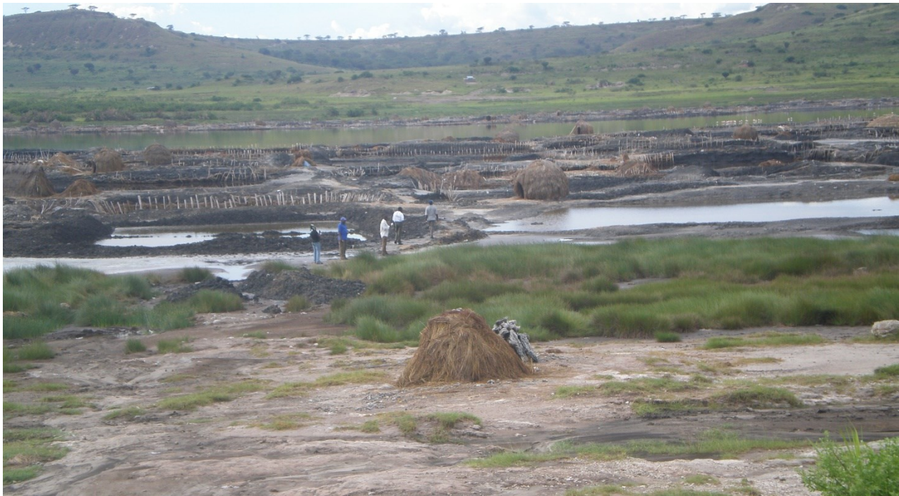
Figure 5: Salt ponds from which the brine from Crater Lake Katwe is concentrated by evaporation using the sunlight energy forming crusts of salt layers that accumulate on pond bottom over time in the dry season.
