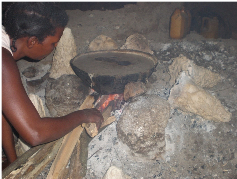
Figure 4: A lady extracting salt at Kibiro geothermal prospect by evaporation to dryness. Note the cones (about 30 cm high) of halite salt made by continuous pouring of precipitated salt. These columns take about 8 hours to extract using dry fire wood collected from the bush around the rift escarpment.
