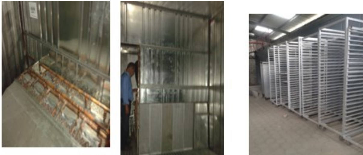
Figure 18: Converted Refrigeration Radiators into to the main Radiator in the dehydration air tunnel. Dehydration trays.
