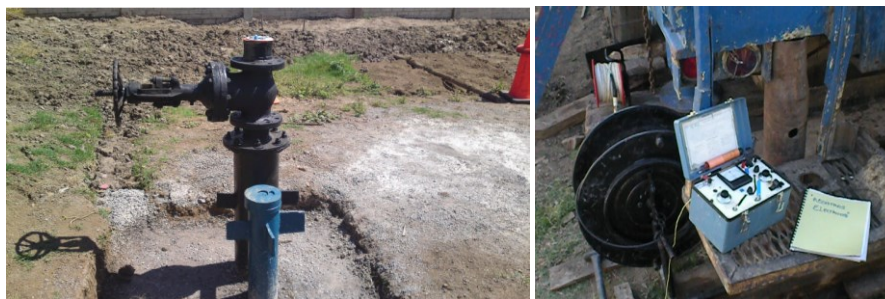
Figure 4: Shallow Exploratory well SM-1, Logging equipment recording SP and Resistivity.
