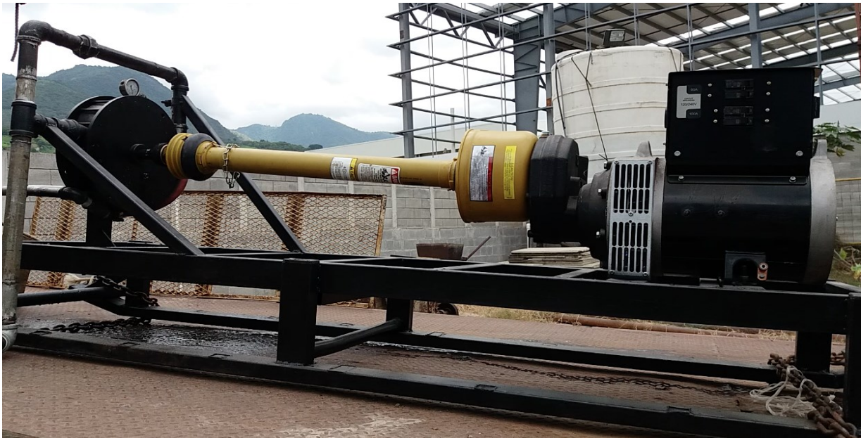
Figure 14: QT5LSC Quasiturbine Attached to the electrical generator.
