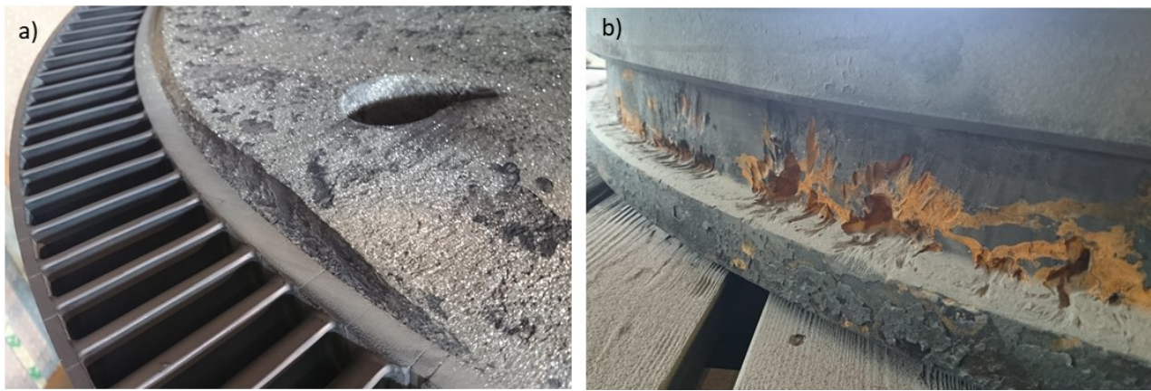
Figure 1: Erosion damages to a) a rotor disc and b) outer edge of a turbine diaphragm.
