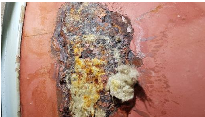
Figure 2: A corroded pipe from ON Power's piping system.
