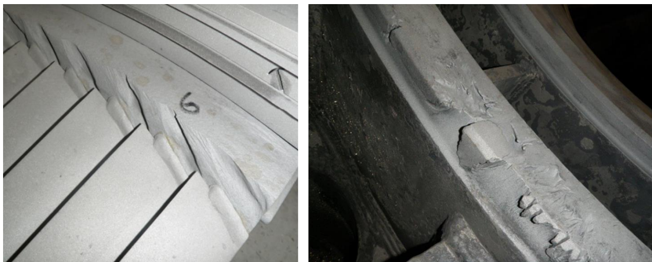
Figure 2: Erosion corrosion in turbine; between blades in the diaphragm (left) and in the casing seat for the diaphragm (right).
