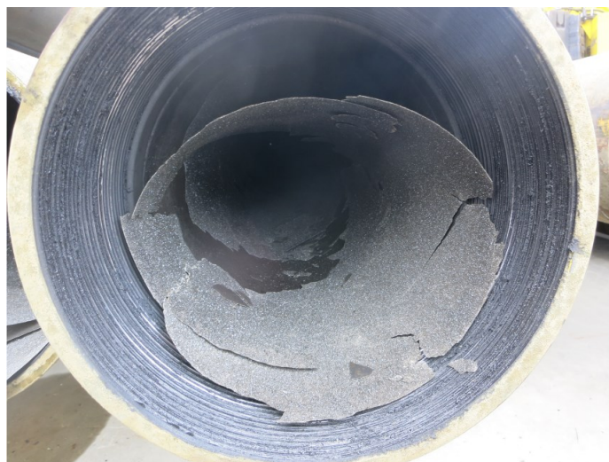
Figure 2: Images of detached precipitates in the production pipe.
