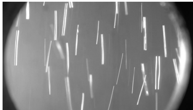
Figure 4: Gas bubbles in the thermal water captured through a porthole at the entrance to the geothermal power plant.
