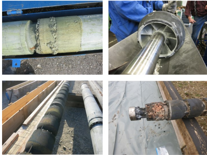
Figure 3: Images of scalings at and inside submersible pumps.
