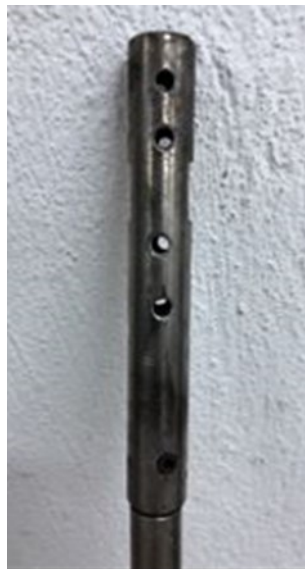
Figure 4. 12 Months Post PCA Treatment implementation coupon clear of Silica deposition
