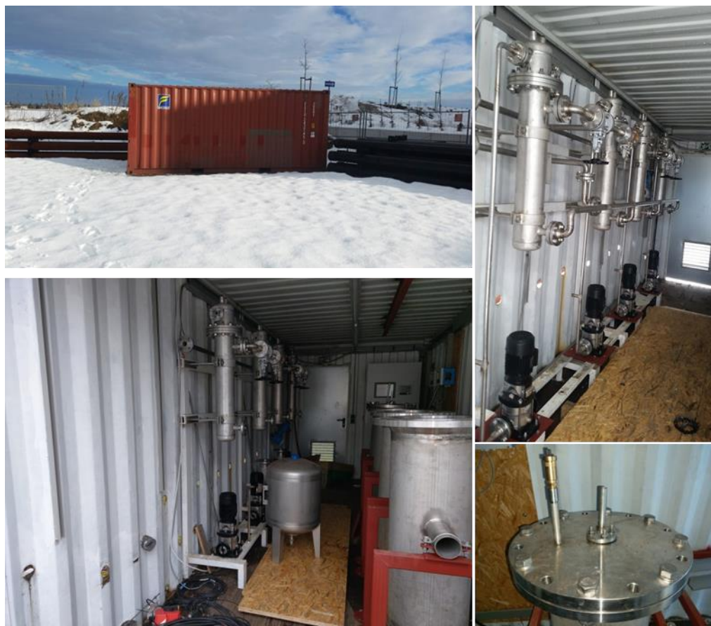
Figure 4: Onsite pilot plant for performing static and dynamic investigation of the stability of the inhibitor and its interactions with the rocks of the geothermal reservoir.
